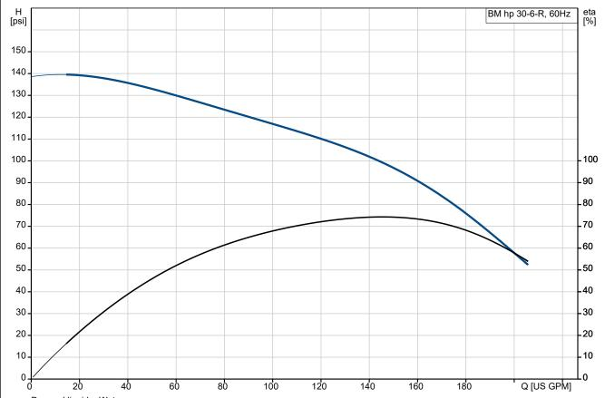
Pumped liquid = Water Liquid temperature during operation = 140 °F
