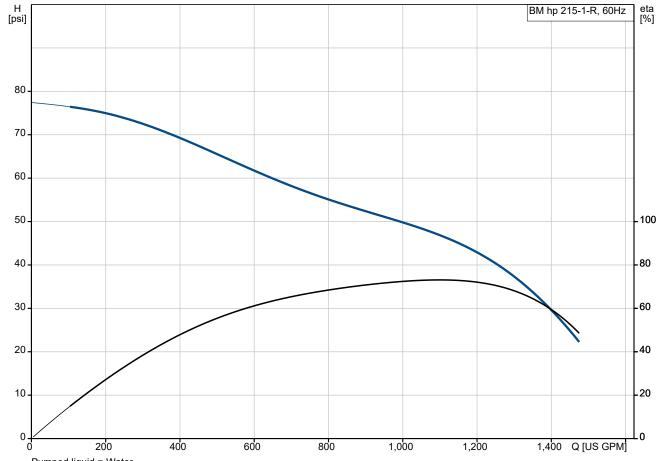
Pumped liquid = Water Liquid temperature during operation = 140 °F
