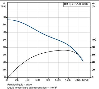
Liquid temperature during operation = 140 °F Density = 61.35 lb/ft³
