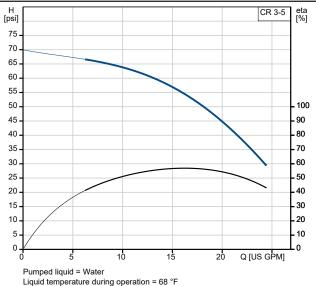
Liquid temperature during operation = 68 °F Density = 62.29 lb/ft³
