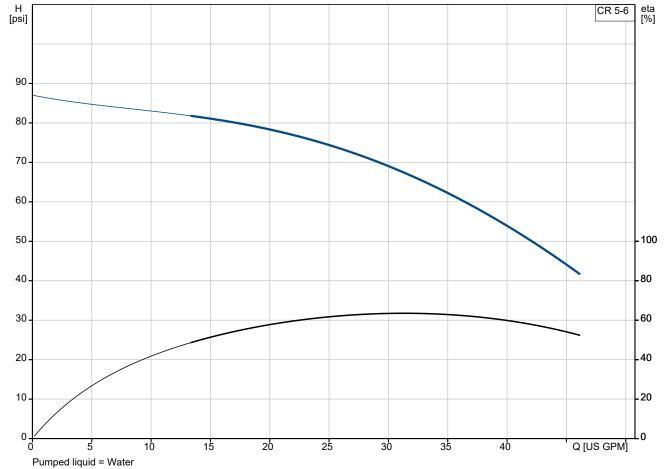
Pumped liquid = Water Liquid temperature during operation = 68 °F
