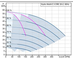
Losses in fittings and valves not included Pumped liquid = Water Liquid temperature during operation = 68 °F Density = 62.29 lb/ft³
