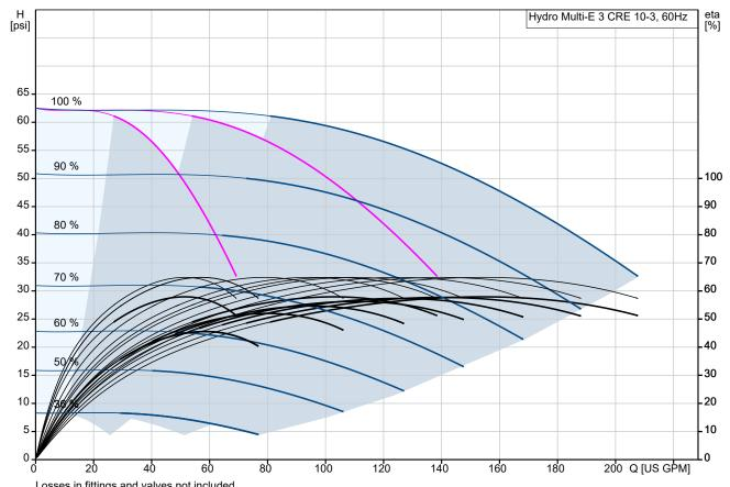
Losses in fittings and valves not included Pumped liquid = Water Liquid temperature during operation = 68 °F
