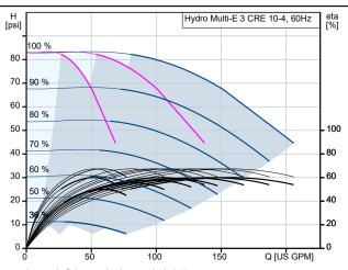
Losses in fittings and valves not included Pumped liquid = Water Liquid temperature during operation = 68 °F Density = 62.29 lb/ft³
