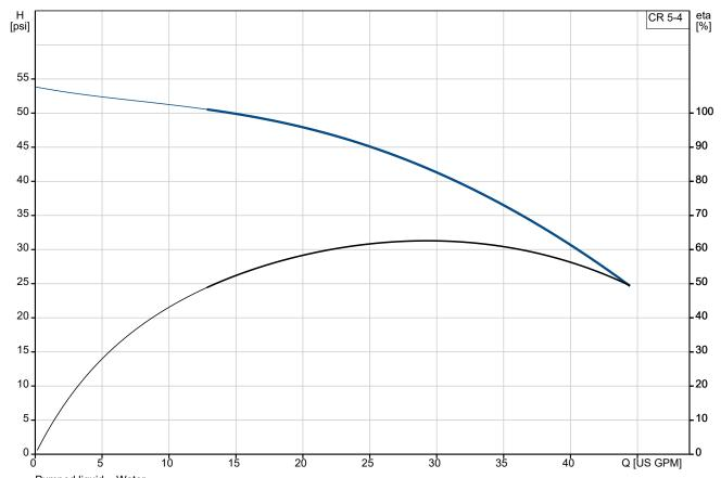
Pumped liquid = Water Liquid temperature during operation = 68 °F Density = 62.29 lb/ft³
