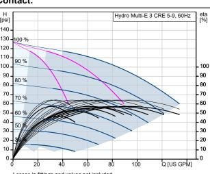
Losses in fittings and valves not included Pumped liquid = Water Liquid temperature during operation = 68 °F Density = 62.29 lb/ft<sup>3</sup>
